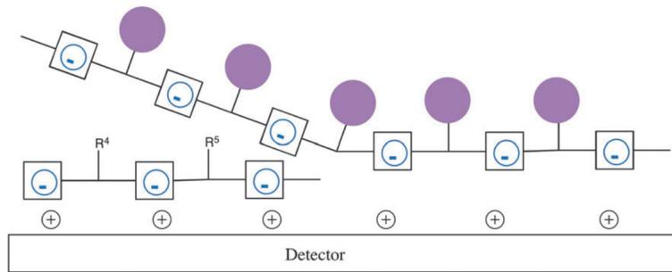
**FIG. 4.** A detector with a repeating positive charge on the surface could detect anionic Darwinian biopolymers in the enceladan geyser, by specific adsorption of the polyelectrolyte polymers onto that surface. A corresponding surface with a repeating negative charge could detect any cationic Darwinian biopolymers that might be in the geyser. Here, detection would be by displacement from the surface of a fluorescently tagged (magenta circles) short polyanionic biopolymer.
