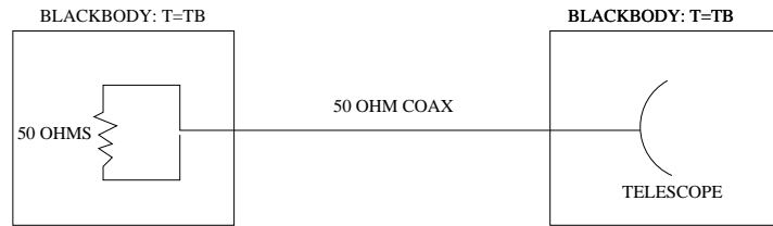
Fig. 2.— A perfectly matched telescope and load, each in its own blackbody cavity; the cavities are at the same temperature.
