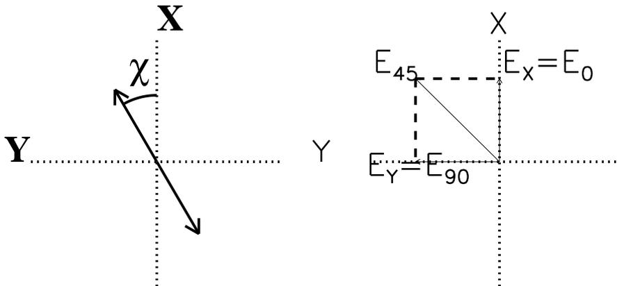
Fig. 1.— Left: The position angle of polarization. Right: Adding  $E_X$  (same as  $E_0$ ) and  $E_Y$  ( $E_{90}$ ) gives  $E_{45}$ .
