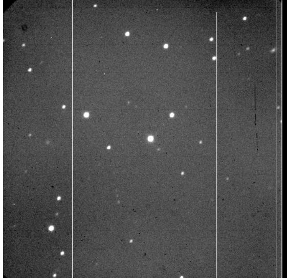
Figure 5: A raw image of a star field obtained with the Direct Imaging Camera (prior to dark subtraction and flat-field correction). The telescope is guiding to keep the target roughly in the center of the image. Many other stars are detected in the image, from which we can select “reference” star to monitor the relative brightness of the target.
