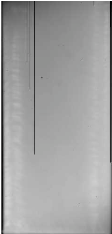
Flat field exposure of an EEV42-80 CCD
